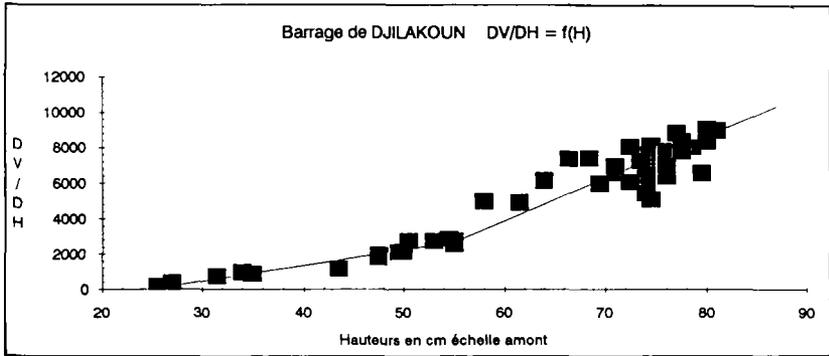
Figure 3. Barrage de Djilakoun.  $DV/DH = f(H)$ .
